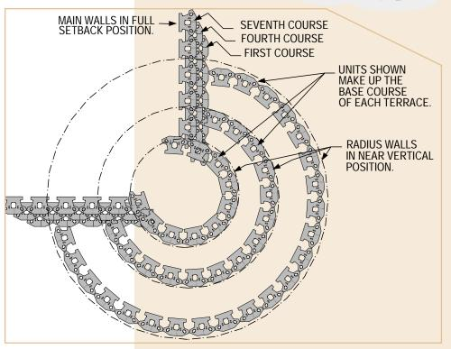
**CORNER DETAIL OPTION** WHEN BUILDING MAIN WALLS IN THE SETBACK POSITION.
