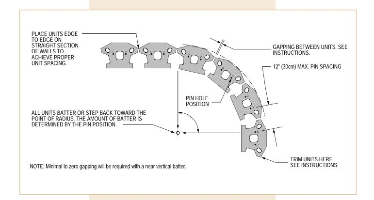
Concave curves are constructed using typical wall units. The following information will provide a complete explanation of construction techniques for building retaining walls with these conditions.
